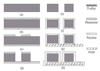
Fig. 3 Process flow of a PVDF-parylene wing.
