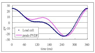
Fig. 7 The "pseudo" signal comes from superimposing a similar curve of Fig. 5(a) with a proper phase lag (11 degree) into Fig. 5(a) itself.
